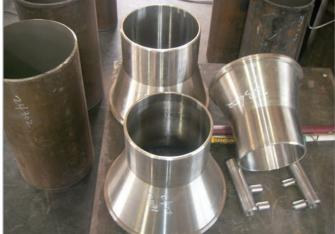
Flow Nozzle is costlier than orifice due to their construction but it is suitable to measure the flow rate of fluid flowing at high temperature and pressure. Under the same measurement condition, the flow nozzle has a higher mechanical strength, can permit the flow of more than 60 percent greater volume of a fluid, and can measure the flow rate of fluid which contains solid particles with less disturbance than an orifice which has the same bore.
