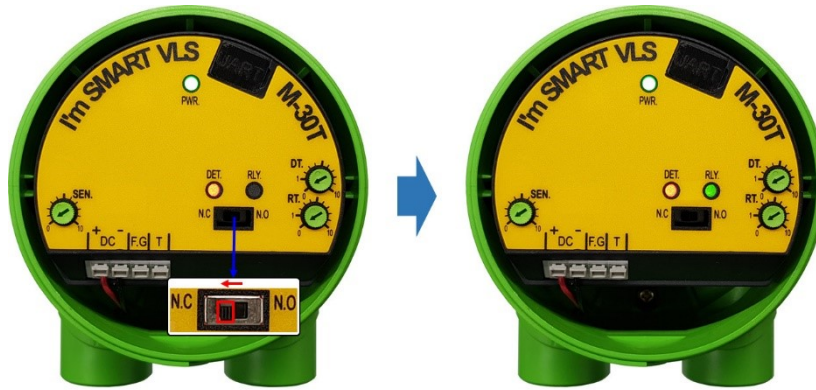
[Operating Status According to Current out [N.C]]
