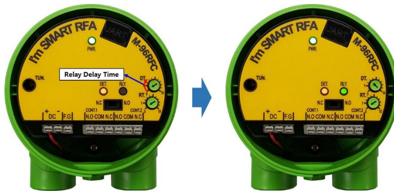
[Operating Status According to Relay Delay Time]
