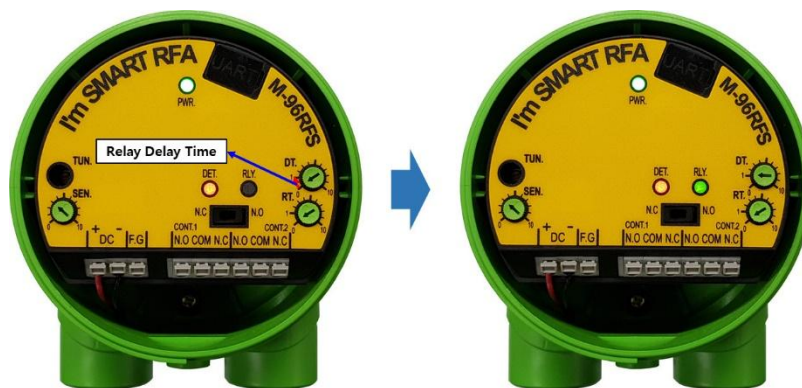
[Operating Status According to Relay Delay Time]
