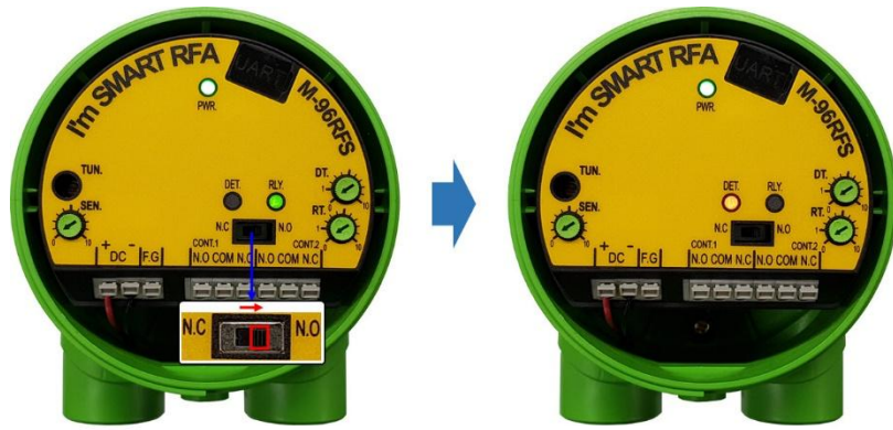
[Operating Status According to Relay Contact [N.O]]
