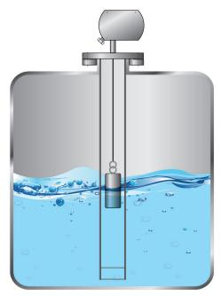
When there is flow or sloshing in the measured object or there is a stirrer around the sensor, the protective tube type should be used.
