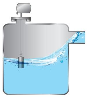
Product should be installed at the place far from inlet in order to avoid the malfunction.
